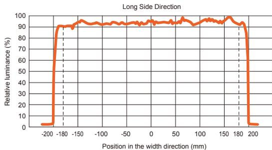
Output of 90% or higher for effective emitting surface of 360 mm.
