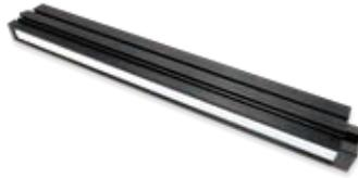
At 400,000 lx, these Light Units represent the brightest class in the industry for natural air cooling. Light diffusion is suppressed with a unique radiation structure to minimize brightness changes for distance. This lets you flexibly set the distance between the inspection object and Light Unit. We can manufacture light-emitting surface lengths from 100 mm to 1,000 mm in 100-mm increments.
